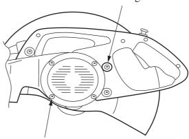
Pan head screws M5(4 pieces) for mounting the motor housing
