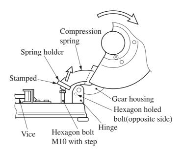
**Note**: The spring holder has a direction. When assembling, arrange in a way that the side with stamped mark may come at vice side.
