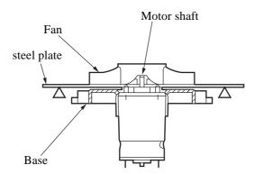
In putting Fan into Motor, be sure to receive the rear end of Motor shaft and put Fan in by pressure so that a gap between Motor and Fan may be  $0.2 \sim 0.7$  mm when Fan is pressed to Motor side.
