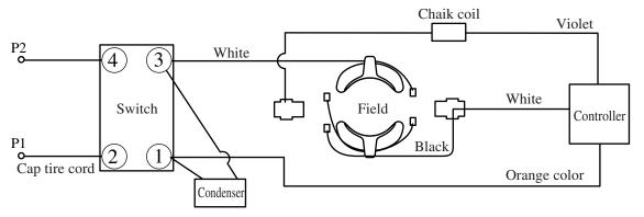
Note: The condenser and chalk coil are not used in some areas. The M434 is only for 100V.
