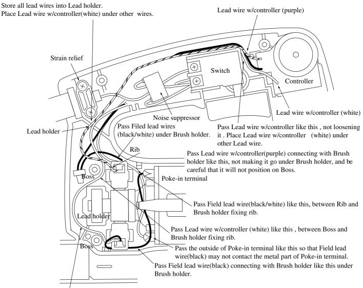
Be careful that Lead wire w/controller(white) will not position on Boss. Push it into the depth of Lead holder.
