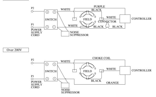
\* Noise suppressor and Choke coil are not used for all counties.
