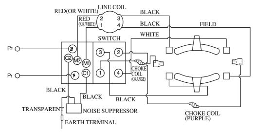
\* Noise suppressor, Line Coil and Choke coil are not used for some counties.
