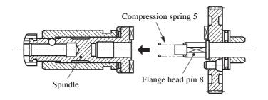
(2) After assembly in the condition of the right illustration, put it into housing.
