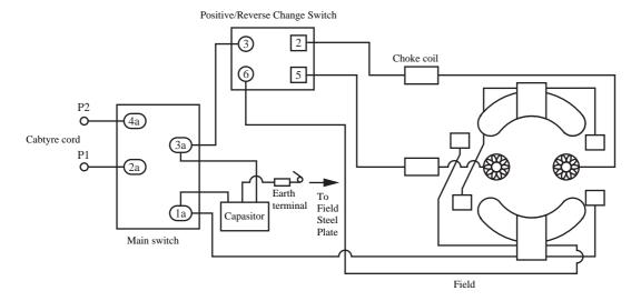
[Note] \* There are some areas where Condenser is not used or where 2-foot condenser(without earth line) is used.
