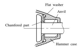
(4) How to dismount the hammer Adjust the open part for steel ball on hammer with the top of groove on spindle pressing the hammer with arbor press. Then the steel ball can be taken off in order to dismount the hammer.
