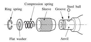
(3) How to mount the flat washer The flat washer has to be mounted between hammer case and anvil. In this case, the chamfered part on the flat washer has to face the anvil as illustrated right.
