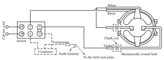
The condenser is not used in some areas and the condenser with two legs(without lead wire) is used in other areas. The chalk coil(with lead wire) is not used in some areas.
