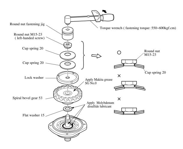
How to exchange Spindle and Ball bearing 6203
