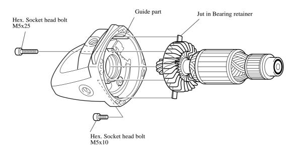
2) How to exchange Spiral gear 12 (16)
