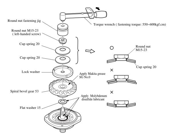
How to exchange Spindle and Ball bearing6203
