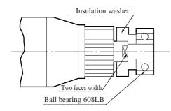
Insert the Insulation washer between the armature commutator side and the ball bearing 608LB. Since both armature shaft and the insulation washer have each two faces width for preventing from turning, be sure to fit these width each other to insert the insulation washer and then insert the ball bearing 608LB in a way that the insulation washer can be fixed using the armature shaft body and ball bearing 608LB.
